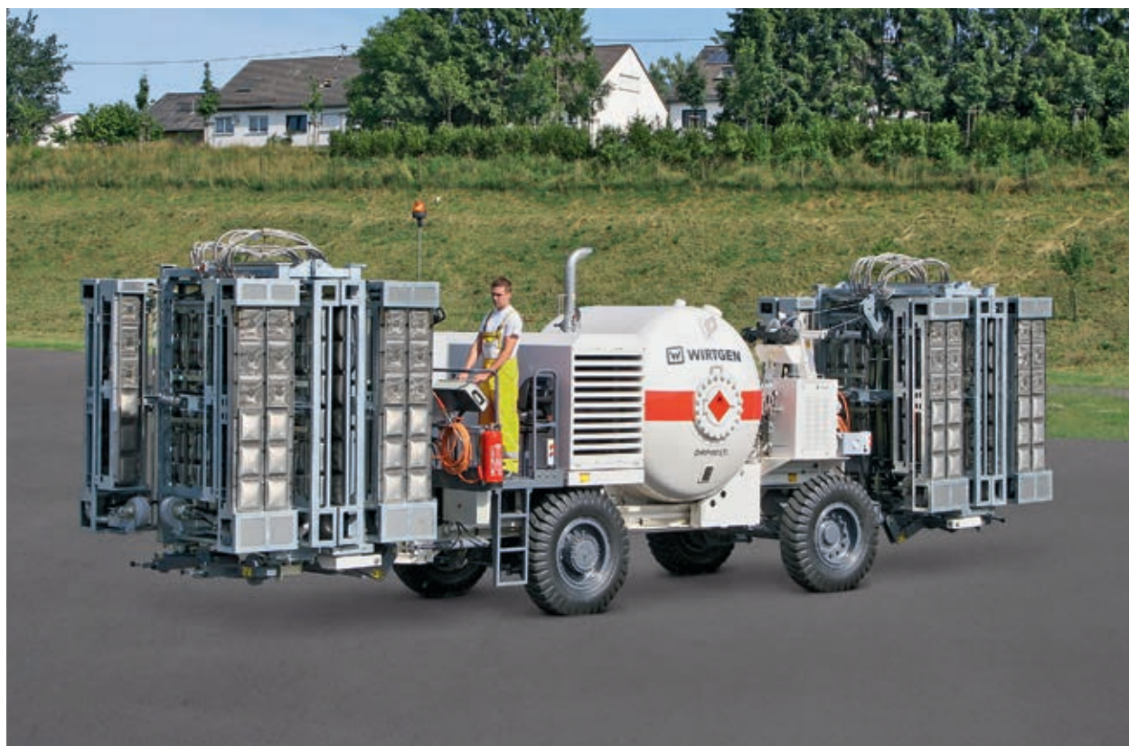
Compact design: the operator simply folds up the heating units for transport.
